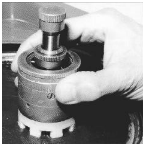
Figure 8.7 (A) Sample holder on the rotating wheel and (B) polishing wheel.
